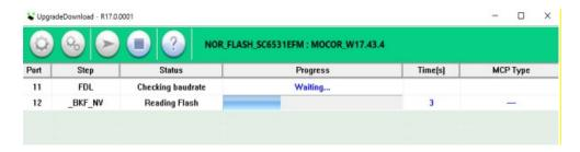
6. After the successful completion of the flashing process in the program interface in the column status you will see the inscription Finish, and in the Progress column - Passed, (you can disconnect the phone from PC and reconnecting the battery to start the device).
